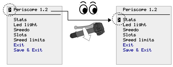
Instead, **to enter into the menu** (or to change a setting) simply rotate the throttle and then <u>release it after a fraction of second</u>.
