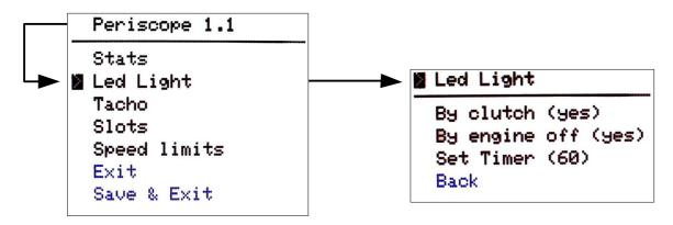
For enabling/disabling first two options you have simply move the cursor over the right command and toggle the value from 'yes' to 'no' (or vice versa). For example:
