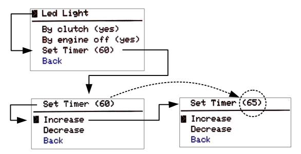
The timer can be useful to save the motorcycle battery if you forget your ignition key on the ON position (with the light ON too).
