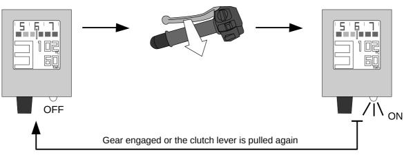
Bike stopped, no gear engaged and theclutch lever is pulled
