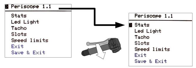
Instead, to enter into the menu (or to execute a command), simply rotate the throttle <u>and</u> then release it after a fraction of second.
