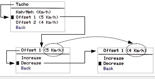
BE SURE THAT THE RIGHT MEASURE UNIT IS SET BEFORE ENTERING TUNING VALUES. If the "tacho" is set to 'Kmh' then the values will be interpreted as an offset in kilometers per hour, or miles per hour otherwise.
