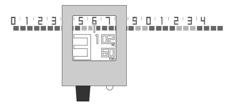
Every tick/bar of the scale indicates a displacement of 5 Kmh (or Mph). The central white tick shows the current speed value.
