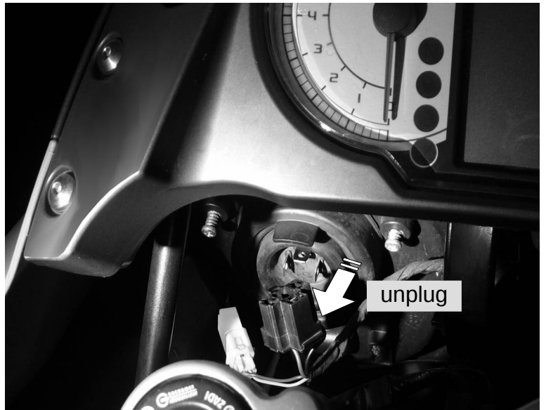
Detach the connector of the left headlamp
