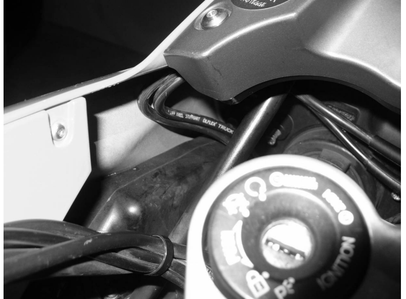
Example: the power cables constrained between the fairing and the metal frame
