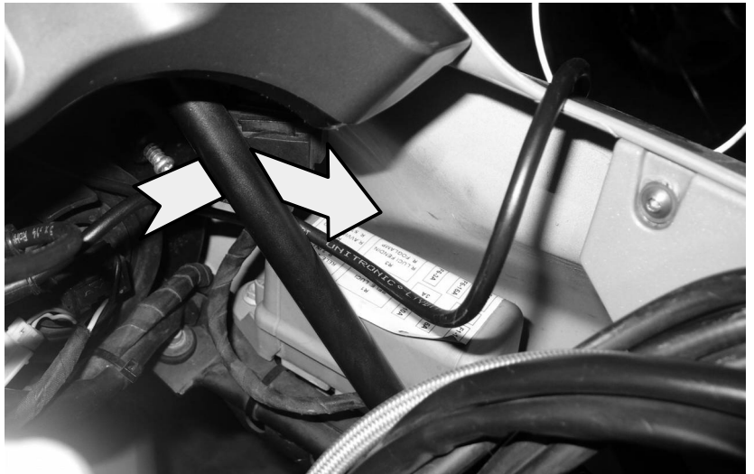
Use the frame pipes to keep the OBD cable away from the fork.
