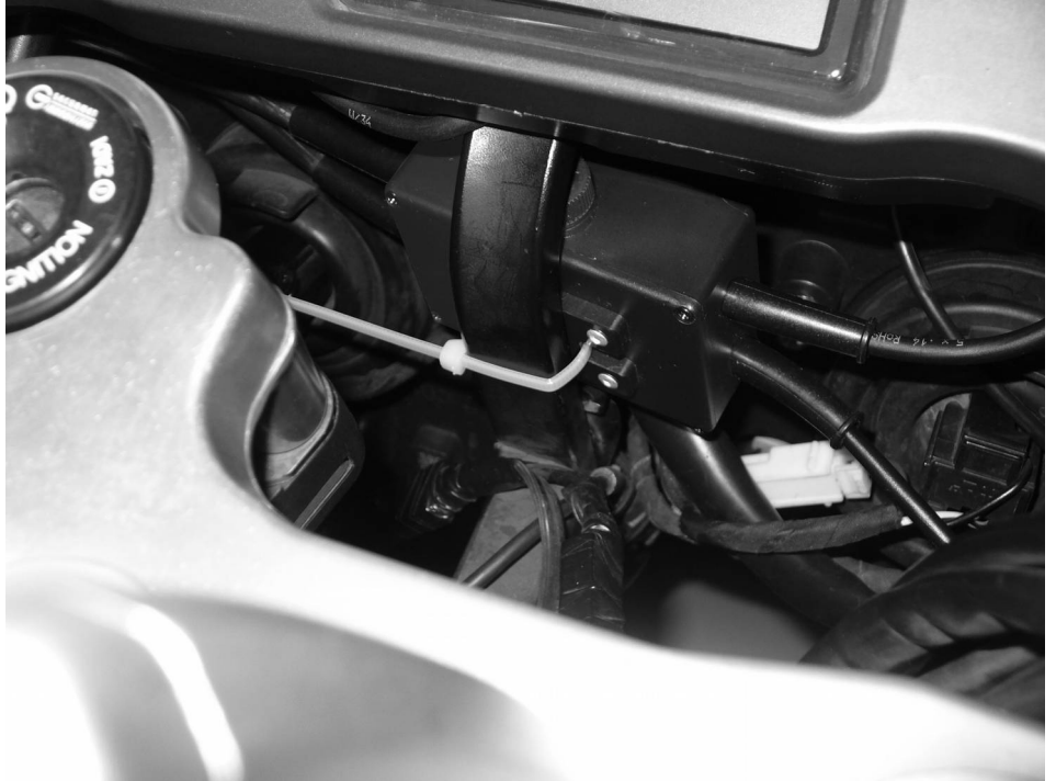
Fasten the decoder unit to the vertical bar
