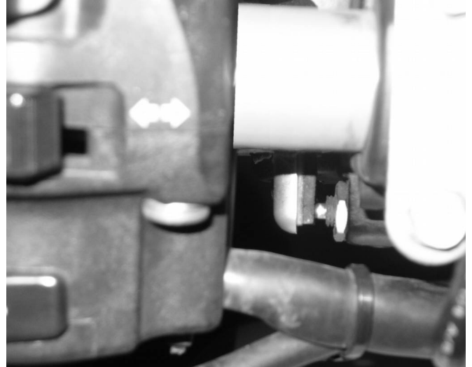
After attaching the pad the micro-switch is activated more promptly and securely.
