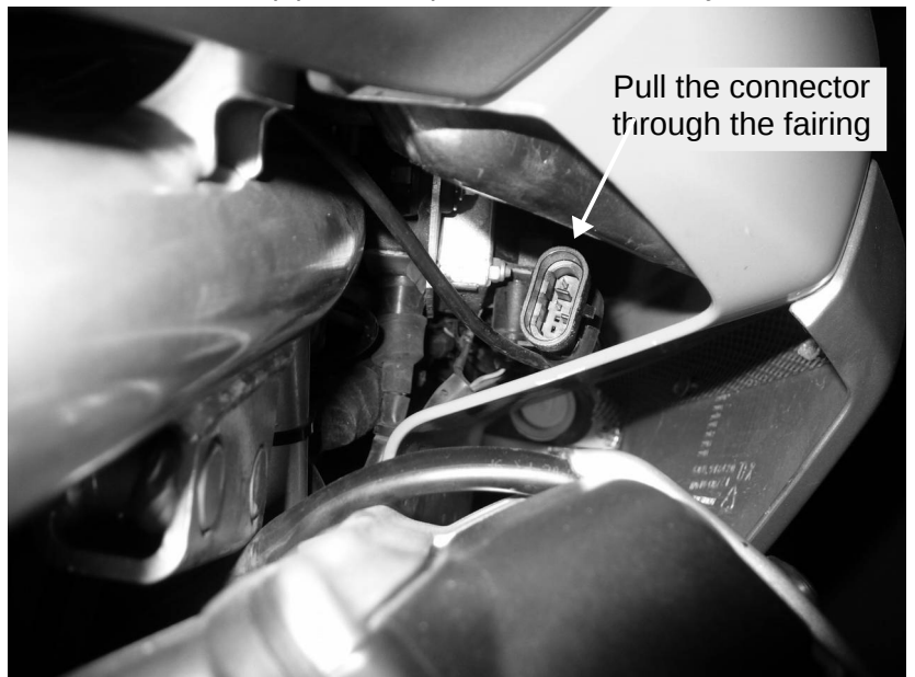
Route the OBD cable through the fairing.
