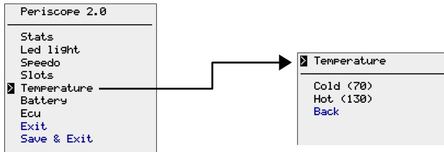
In the example below the upper threshold is increased by 5 Celsius degrees:
