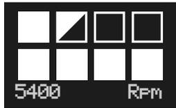
It shows the current RPM value by using two little rows composed of four bars.
