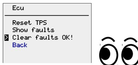
4. Pull the clutch to return back at the **Ecu** menu, or simply turn off the ignition key.
