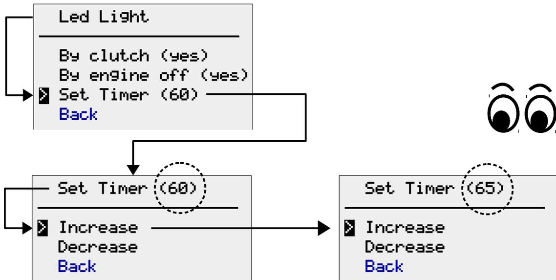
The timer can be useful to save the motorcycle battery if you forget your ignition key on the ON position (with the light ON too).
