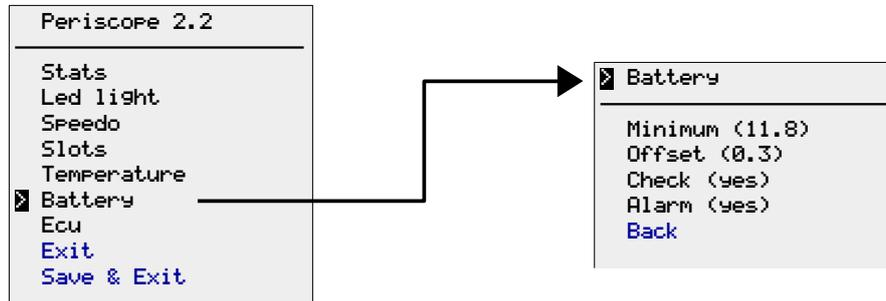
When displayed, the indicator will start flashing when the voltage level goes down the **Minimum** level. You can increase/decrease the level by moving the cursor over the item and selecting it.
