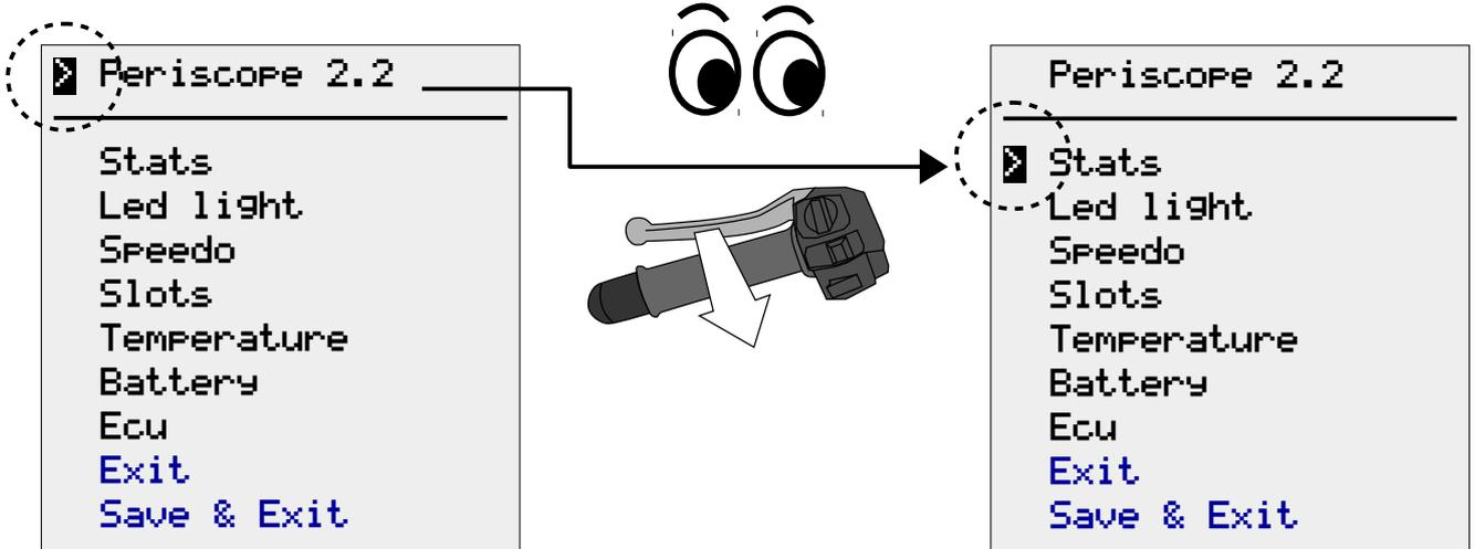
Instead, to **enter into the menu** (or to change a setting) simply rotate the throttle and then release it after a fraction of second.
