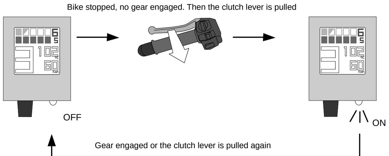
Note: if the engine is running, and you engage a gear, then the light will be automatically turned off.
