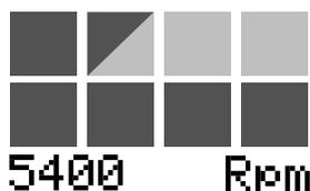
It shows the current RPM value by using two little rows composed of four green bars.
