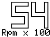
Shows the current RPMs of the engine as a number. RPMs are divided by 100.
